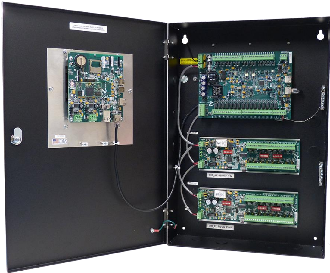
Figure 3 TELSEC ESB2x Inside Panel
