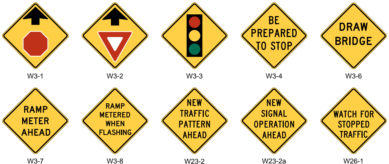
Figure 2C-8. Advance Traffic Control Signs
